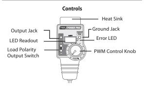
CAUTION! The Heat Sink can become extremely hot during use. Therefore, avoid contact with your skin or any of the vehicle's components.
