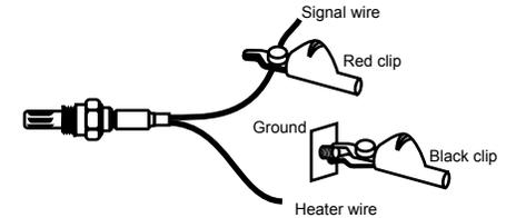
Three wire (heated) sensor
