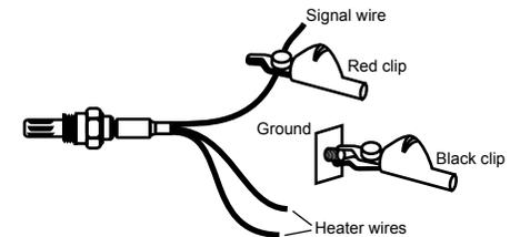
Four wire (heated) sensor
