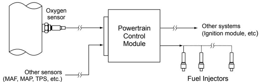
Fig. 4 - Oxygen sensor function
